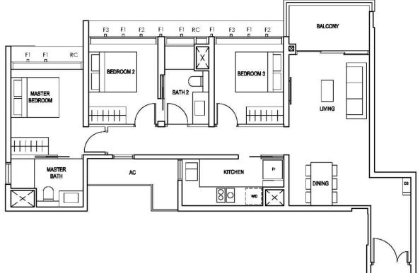
FULL HEIGHT ALUMINIUM FIN LOCATED AT LEVELS: F1 - #03 to #18 F2 - #05, #06, #09, #10, #13, #14, #17 & #18 F3 - #03, #04, #07, #08, #11, #12, #15 & #16
